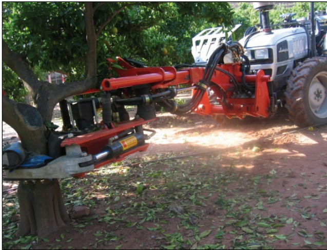
Figure 1. Tractor-mounted trunk shaker used in field experiments.
