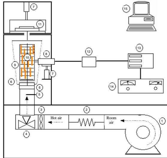
**Figure 1.** Convective dryer. (1) Fan; (2) Heating; (3) Anemometer; (4) Pneumatic three-way valve; (5) Temperature probe Pt-100; (6) Coupling material; (7) Elevator; (8) Ultrasonic transducer; (9) Braces; (10) Parallel plate support; (11) Scale; (12) Impedance matching unit; (13) Digital wattmeter; (14) Generator of power ultrasound; (15) Computer-controller.
