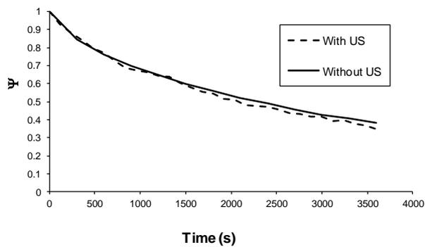
**Figure 4.** Experimental drying kinetics at 40 °C and 1m/s with and without ultrasound application
