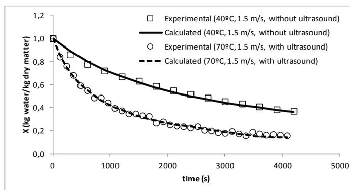
**Figure 5.** Comparison between modeled by Peleg's model and experimental drying curves for two drying conditions (40°C, 1.5 m/s, without ultrasound and 70°C, 1.5 m/s, with ultrasound)
