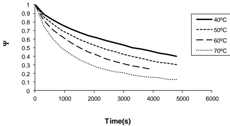
**Figure 2.** Experimental drying kinetics at different temperatures and an air velocity of 1 m/s (without ultrasound application)
