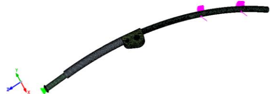
Figure 4. Finite element model of the GSDyn with 2 rib hooks and hence 2 lateral static forces simulating scoliotic curvatures in the frontal plane of the patient.
