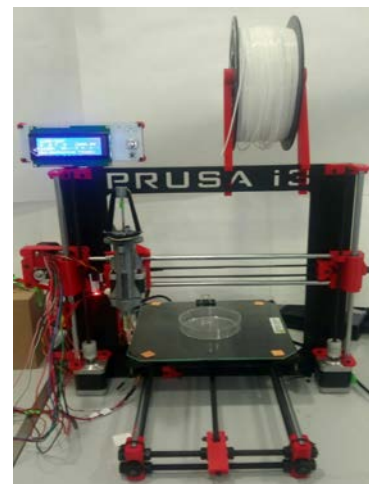
Figure 5. Functional Bio-printer resulting from the integration of the mounted 3D printer Prusa i3 Hephastos with the previously assembled syringe pump (Figure 1) embedded in the X-axis.
