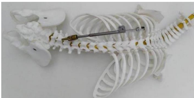
Figure 14. First prototype of GSDyn device assembled to a 5 year old scoliotic spine replica.
