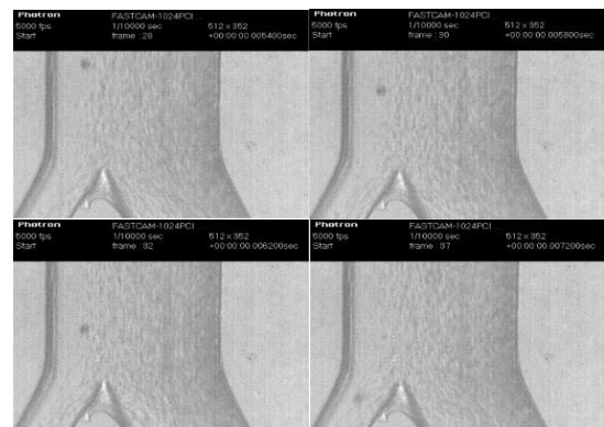
Figura 3. Stacked images showing the movement of a particle in the bifurcation of the device. It can be clearly appreciated how it is separated from the main part of the blood cells.
