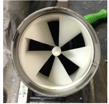
Figure 8.7: Image of the 3D-printed IGV device fitted to the compressor inlet duct, looking towards the impeller.
