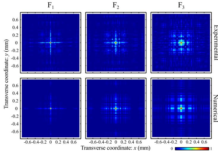
Fig. 5. Experimental transverse irradiance (top) compared with the analytically obtained irradiance (bottom) for a fractal order  $S = 3$  CDZP. Transversal planes belong to the first order focus shown in Fig. 4(b) located at  $z = 10.4$  cm and two secondary foci at  $z = 11.3$  cm and  $z = 13.6$  cm.
