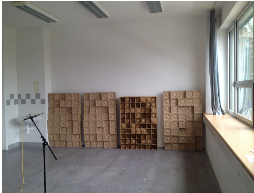
FIGURE 4.19: Distribution of the diffusers in the class room 202a
