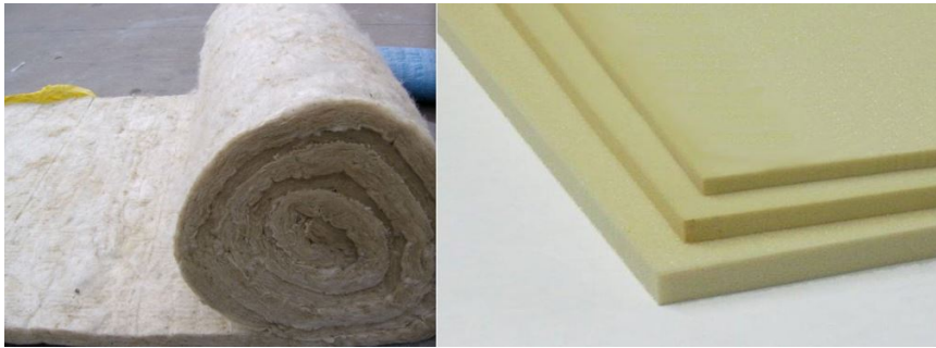
FIGURE 4.13: Rockwool (left) and polyurethane foam (right)
