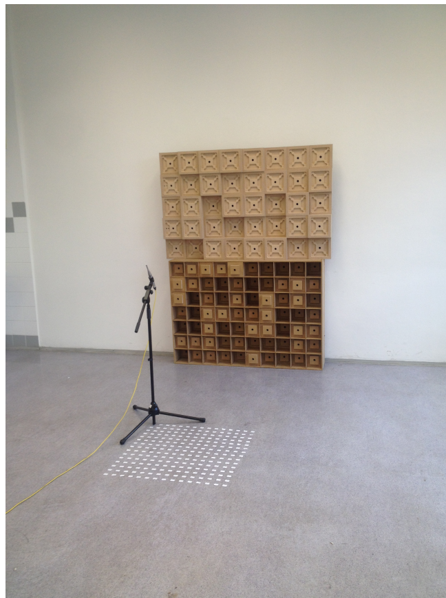
FIGURE 4.16: Passing the microphone over all the points of the grid of the class room 205
