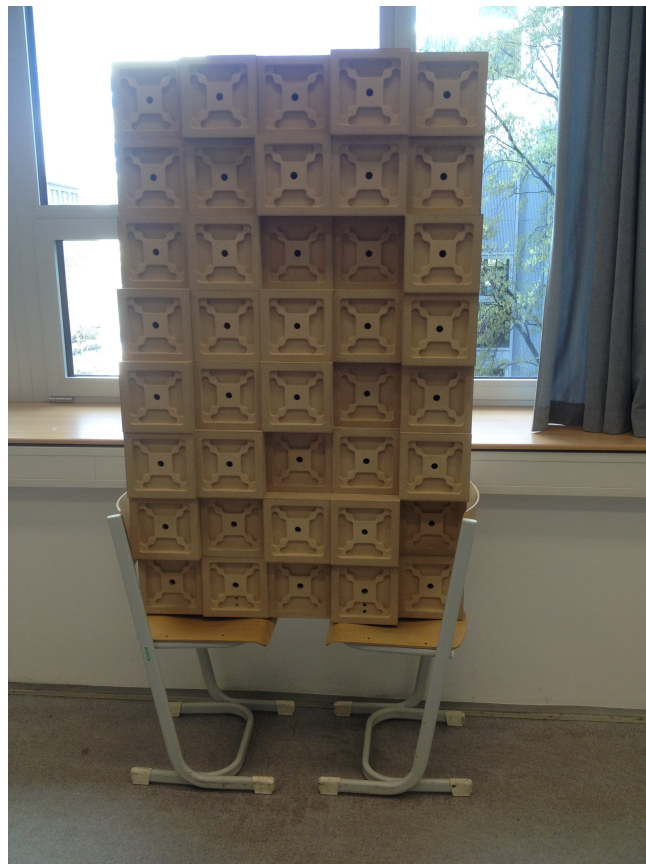
FIGURE 4.15: close look to one of the diffusers
