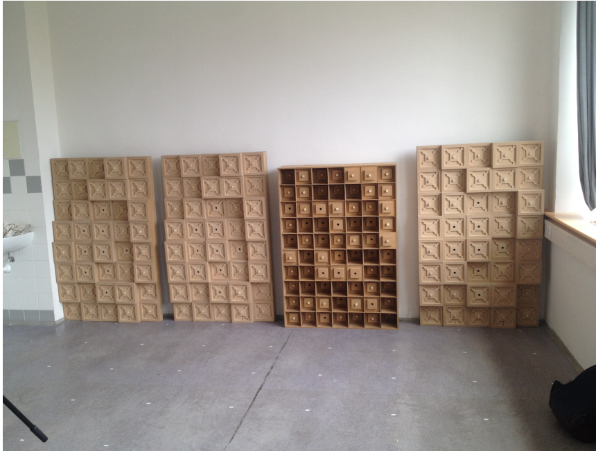
FIGURE 4.14: Diffusers used for the measurements
