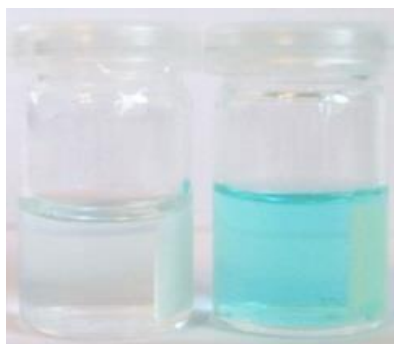
Figure 5. Photograph of a 1.0 cm x 2.0 cm silica dipstick immersed into 2 ml of PBS (0.01 mM, pH 7.0) and with 0.18 ml of SQ (acetonitrile, 1.0 \times 10^{-4} M). The right-hand stick was previously immersed into formaldehyde (1 mM) for 5 min, whereas the left-hand foil was directly immersed into PBS-SQ solution.
