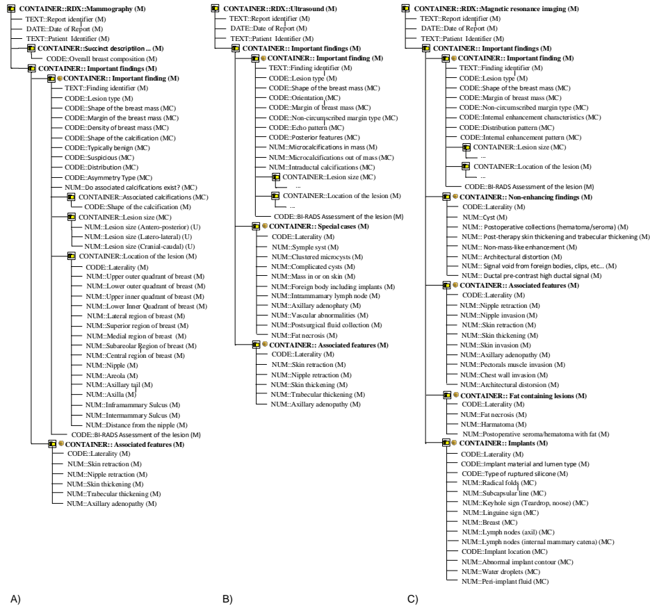
Figure 6. Basic tree of DICOM-SR templates for the three modalities: A) mammography, B) ultrasound and c) MRI.
