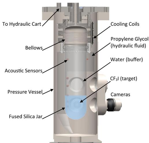
FIG. 1. A schematic of the PICO-60 bubble chamber.
