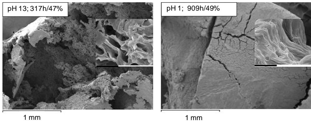
Figure 4. Superficial SEM microphotographs of samples at different degradation times for samples degraded at pH 13 after 317 h and 47% of weight loss (left) and at pH 1 after 909 h and 49% of weight loss (right). The insets show a higher magnification (bar=10µm)
