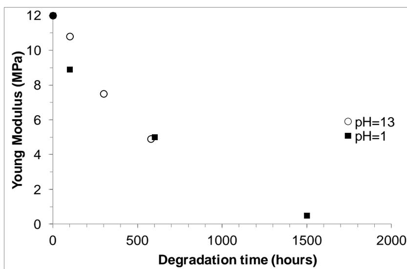
Figure 7. Young's modulus of films degraded at pH 13 and pH 1 as function of degradation time.
