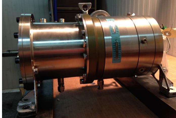
Fig 2. Swash-plate expander delivered by Exoès
