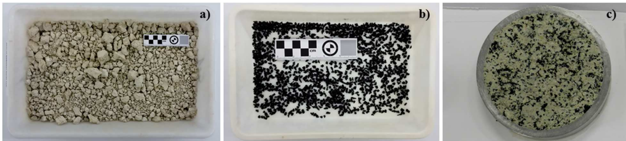
Fig. 1. Soil and rubber samples: (a) Soil; (b) Rubber particles; (c) Soil-rubber mixture (Scale bar in cm).
