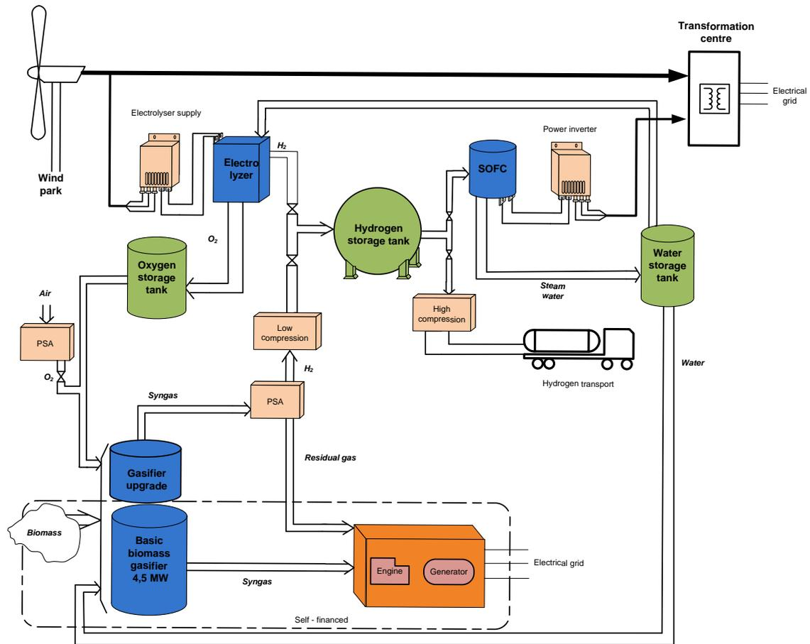
Figure 1: Diagram block of the complete system.
