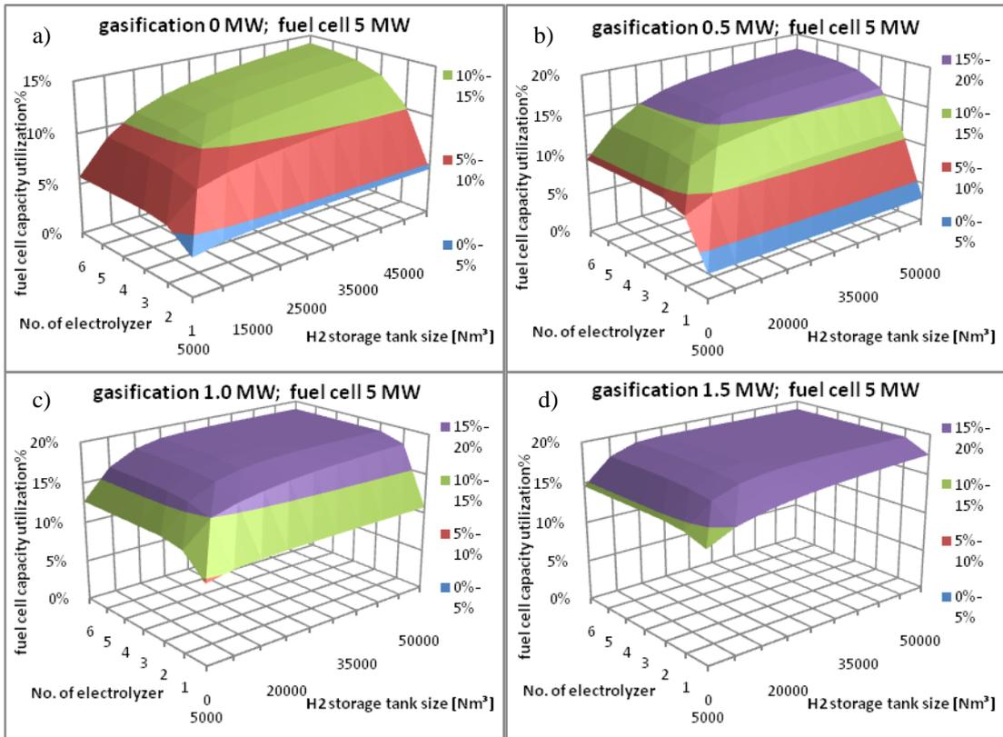
**Figure 5:** Fuel cell capacity utilization for different biomass upgrade gasifier power: a) 0 MW, b) 0.5 MW, c) 1 MW and d) 1.5 MW, with 5 MW fuel cell set power. Scenario number 1: 12/12.
