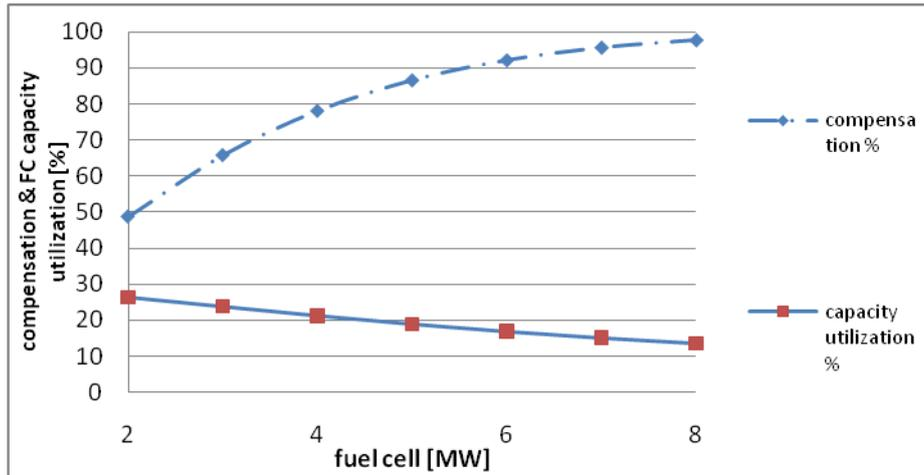
**Figure 3:** Maximum compensation factor and fuel cell's capacity utilization factor for different fuel cell power in the scenario number 1: 12/12.
