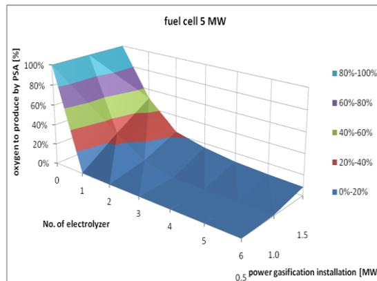
**Figure 8:** Percentage of oxygen produced by the PSA system from the air that gasifier need, for different biomass upgrade gasifier power and number of electrolyzers, with 5 MW fuel cell set power. Scenario number 1: 12/12.
