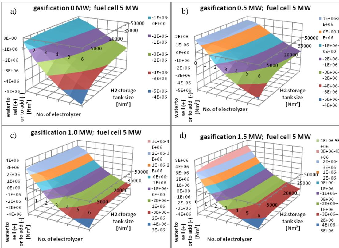
**Figure 7:** Flow of water in the system (excess is positive and defect is negative) for different biomass upgrade gasifier power: a) 0 MW, b) 0.5 MW, c) 1 MW and d) 1.5 MW, with 5 MW fuel cell set power. Scenario number 1: 12/12.
