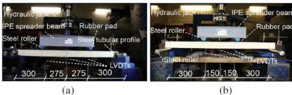
Fig. 9. Test setup for four-point bending tests up to failure of specimens: (a) with GFRP ‘U’ profile (P1U and P2U); (b) without GFRP ‘U’ profile (P1 and P2) (all units in millimetres).
