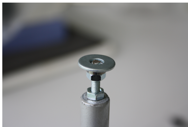
Figure 6. Detail of the washer-ball bearing assembly supported by the nut, without the arm.
