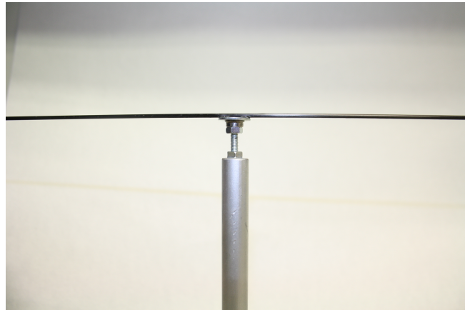
Figure 5. Arm assembly in the endless screw supported by the upper nut.
