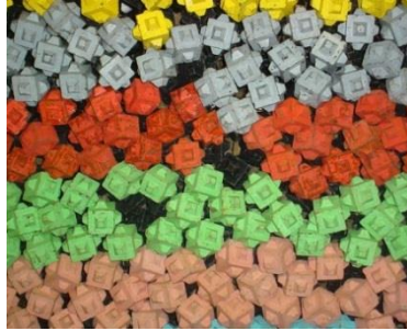
Figure II.8. View of IDa for double-layer Cubipod armor.
