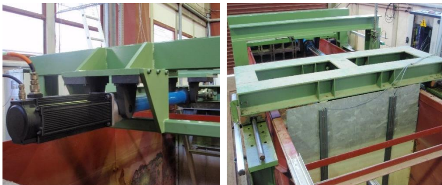
Figure III.3. Piston-type wavemaker used in the experiments.
