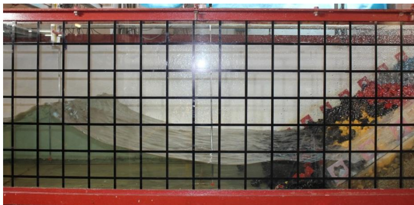
Figure III.10. View of test conducted with breakwater model.
