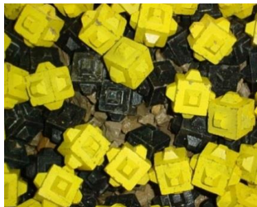
Figure II.10. View of IDe for double-layer Cubipod armor.
