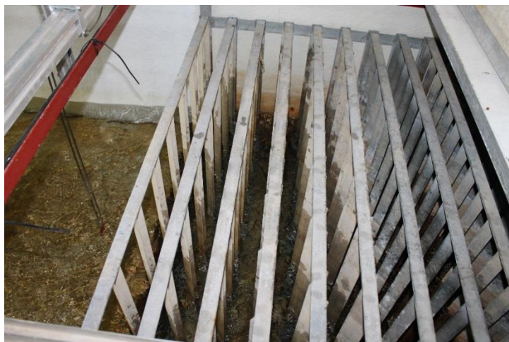
Figure III.4. Passive energy absorber system used in the experiments.
