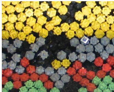
Figure II.9. View of IIDa for double-layer Cubipod armor.
