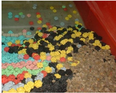
Figure II.11. View of De for double-layer Cubipod armor.
