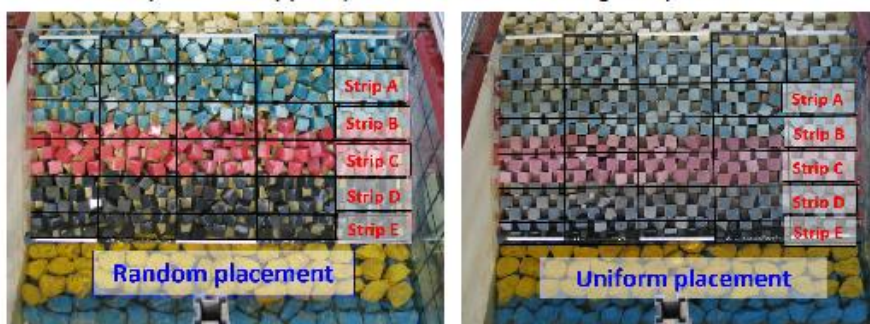
Figure 5. Application of the Virtual Net method proposed by Gómez-Martín and Medina (2014) to measure armor damage in the experiments.
