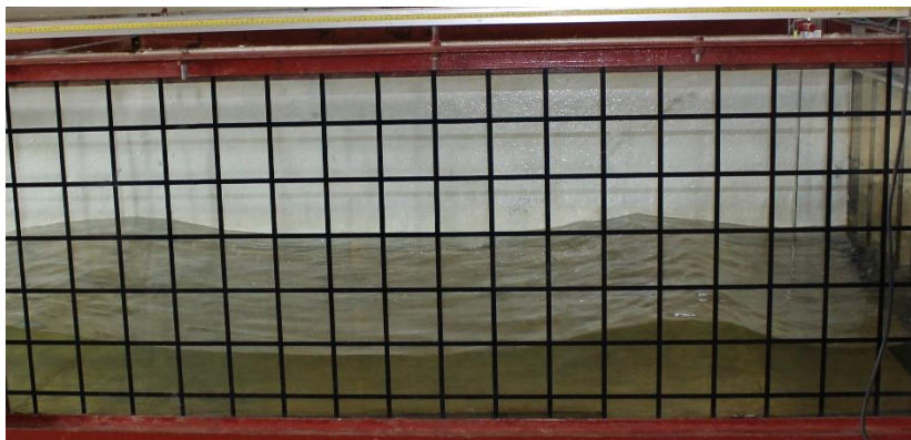
Figure III.11. View of test conducted without breakwater model.
