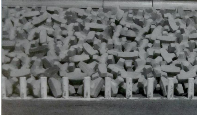
Figure II.17. Toe using concrete piles (CIRIA/CUR/CETMEF, 2007).
