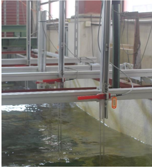
Figure III.12. Capacitive wave gauges used in the experiments.
