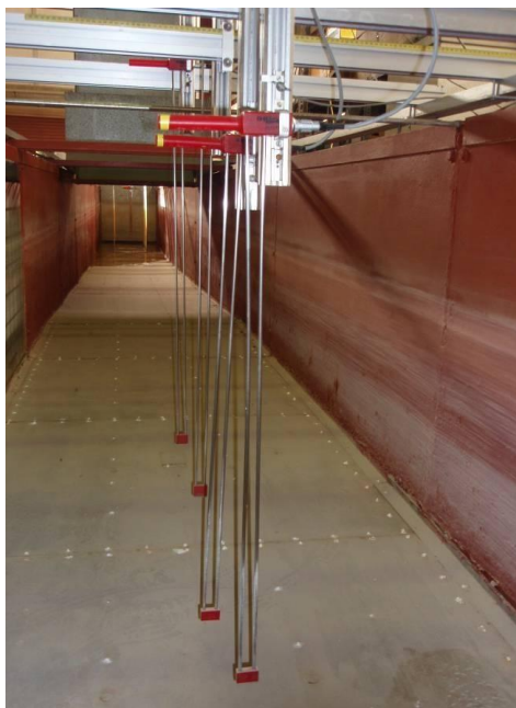
Figure IV.10. Wave gauges located in the model zone.
