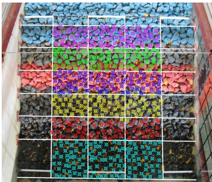
Figure III.15. Virtual net used in the experiments to characterized armor damage.
