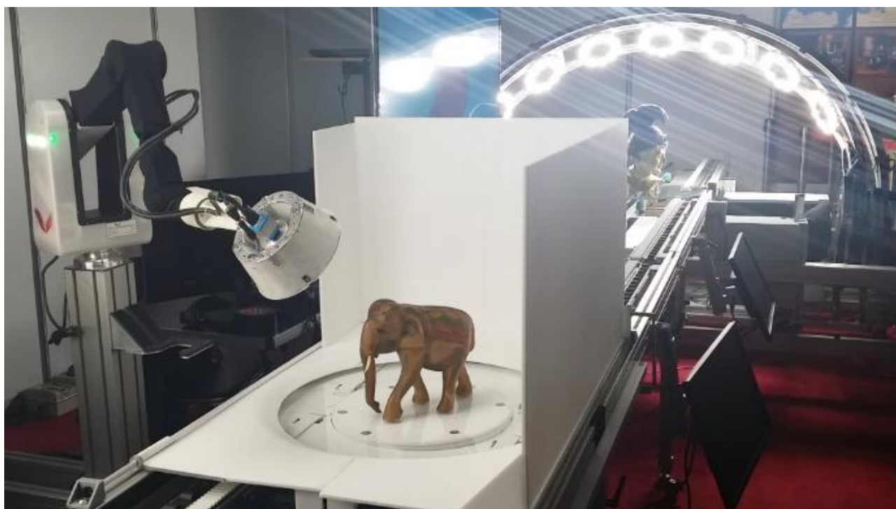
Figure 4: CultArm3D, part of CultLab3D at Digital Heritage 2015 in Granada, Spain. CultArm3D is used to resolve remaining occlusions or holes not covered by the first scanning station CultArc3D.
