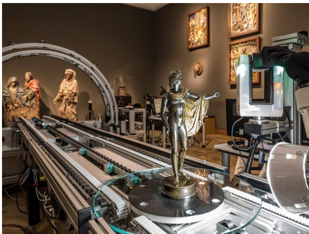
Figure 2: Fraunhofer IGD's CultLab3D pipeline system at the Liebieghaus Skulpturensammlung. "Apollo Belvedere" (1497/98) by Renaissance sculptor Pier Jacopo Alari Bonacolsi (ca. 1460-1528), called Antico, on the mobile digitisation lab. Liebieghaus Skulpturensammlung's Medieval Hall. Photograph: Norbert Miguletz © Liebieghaus Skulpturensammlung.
