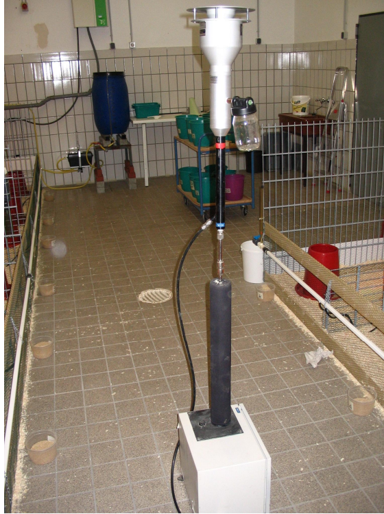
Figure 6.5. Particulate matter sampling device for PM 10 (TEOM)
