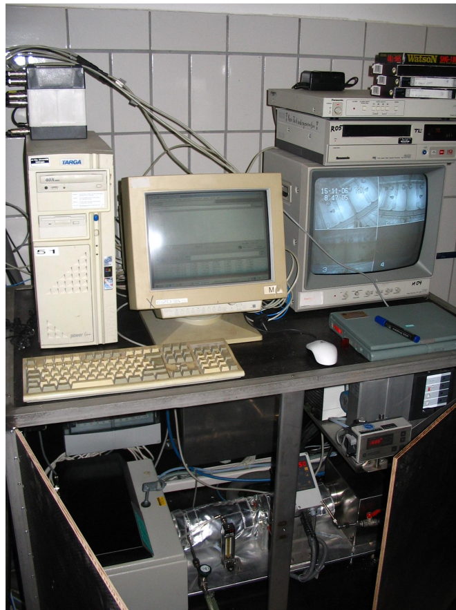
Figure 6.4. Video recording system and FTIR multi-gas analyzer
