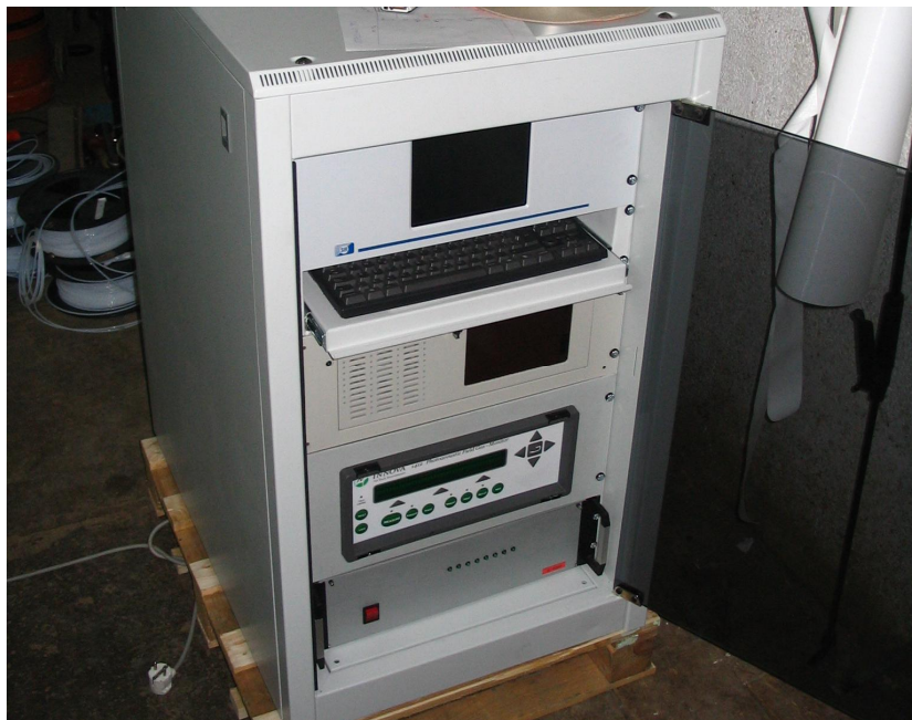
Figure 4.4. Gas measurement system including the photoacoustic gas monitor, a pneumatic multiplexing system and a computer for data logging
