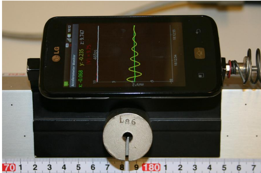
Figure 5. Photograph of the smartphone displaying an acceleration graph for the case of damped oscillations
