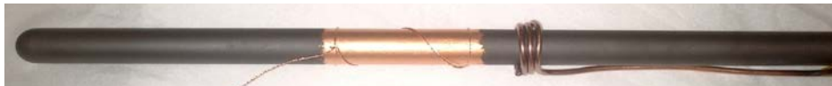
Figure 125. Picture of the reduced BZCY72 TM-1 with the copper anode sintered (anode length \sim 4 cm).
