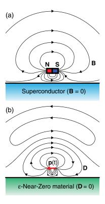
FIG. 1 (color online). ENZ analog to perfect diamagnetism. Analogy between (a) the Meissner effect and (b) the levitation of an electric radiating dipole source over an  $\varepsilon$ -near-zero (ENZ) substrate.
