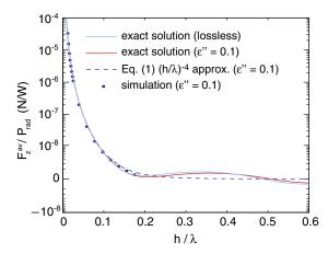
FIG. 3 (color online). Repulsive force dependence on height. Plot of the normalized time-averaged force acting on a horizontal electric point dipole over an ENZ substrate as a function of the normalized height using independent calculation methods: exact solution, near-field approximation, and numerical modeling.
