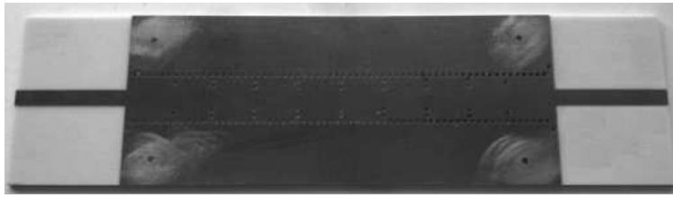
Fig. 4. Manufactured SIW 8 coupled-cavities filter
