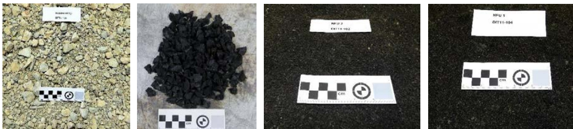
Figure 1. Subballast and rubber samples. (a) Unbound Granular Material-Subballast (b) Rubber 20 mm. (c) Rubber 2 mm. (d) Rubber 1 mm.
