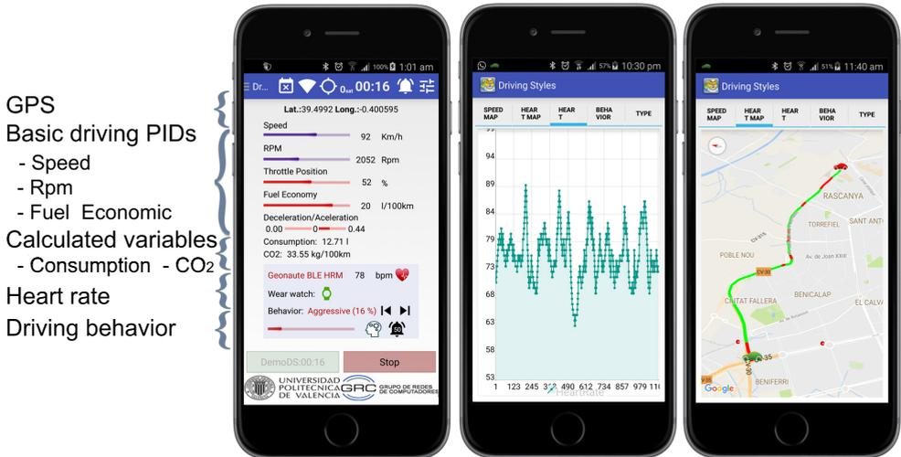
**Figure 7.3:** Snapshots of the main screen and the heart rate module for the Android application.
