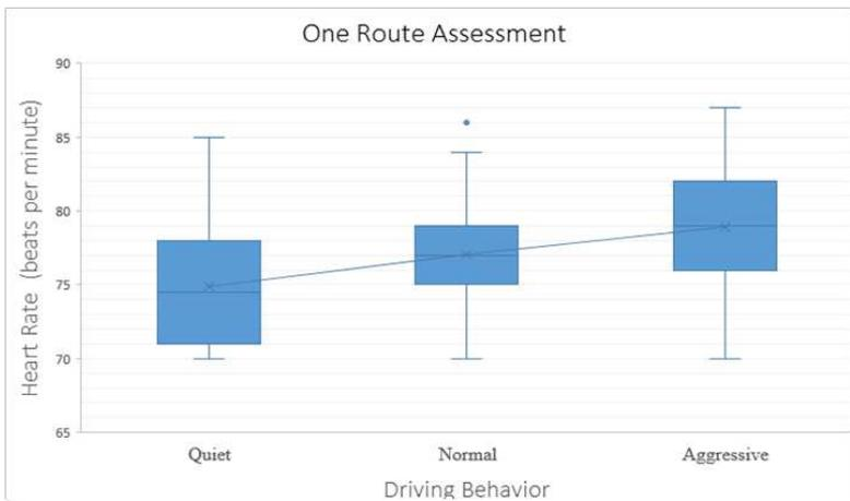
**Figure 6.8:** Box and whisker plot of heart rate vs driving behavior.
