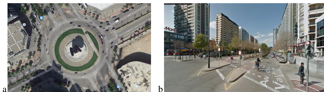
Figure 4. Roundabout in Valencia. Figure 4a. Aerial view of the roundabout: in NW direction, Avenida de las Cortes Valencianas (111 m wide, 7 traffic lanes in each direction), in NE direction, Carrer de la Safor (70 m wide, 5 traffic lanes in each direction). Figure 4b. NW section of Avenida de las Cortes Valencianas. Source: Google Street View (accessed on 20 th October 2014).
