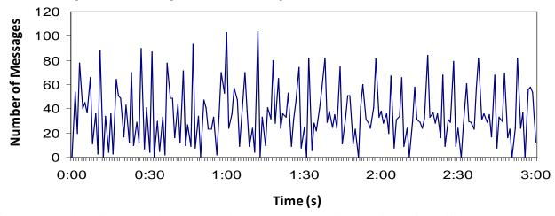
Figure 17. Number of messages observed when the network converges in Scenario 2, using default parameters.
