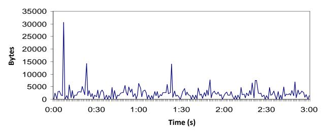
Figure 19. Number of Bytes observed when the network converges in scenario 2, using modified parameters.
