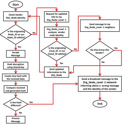
Figure 7. Secure system for data transmission.
