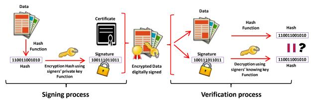
Figure 6. Process of singing, encrypting and decrypting the data using hash and private key function
