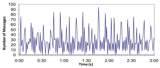
Figure 14. Number of messages observed when the network converges in Scenario 1, using modified parameters.
