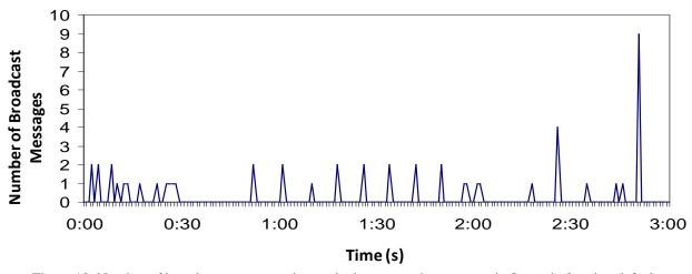
Figure 18. Number of broadcast messages observed when network converges in Scenario 2, using default parameters.
