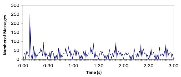
Figure 20. Number of messages observed when network converges in scenario 2, using modified parameters.
