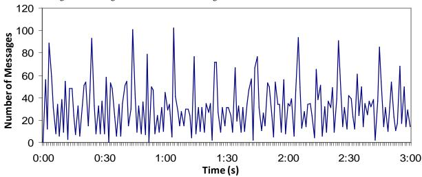
Figure 11. Number of messages obtained when the network converges in Scenario 1, using by default parameters.
