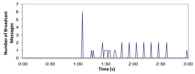
Figure 12. Number of broadcast messages when network converges in Scenario 1, using default parameters.
