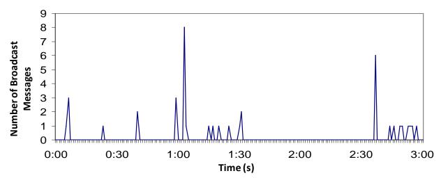
Figure 21. Number of broadcast messages observed when network converges in scenario 2, using modified parameters.
