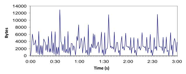
Figure 16. Number of Bytes observed when the network converges in Scenario 2, using default parameters.
