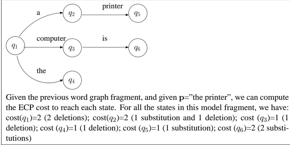
**Figure 3.7:** Example of error prefix correcting parsing on a word graph fragment
