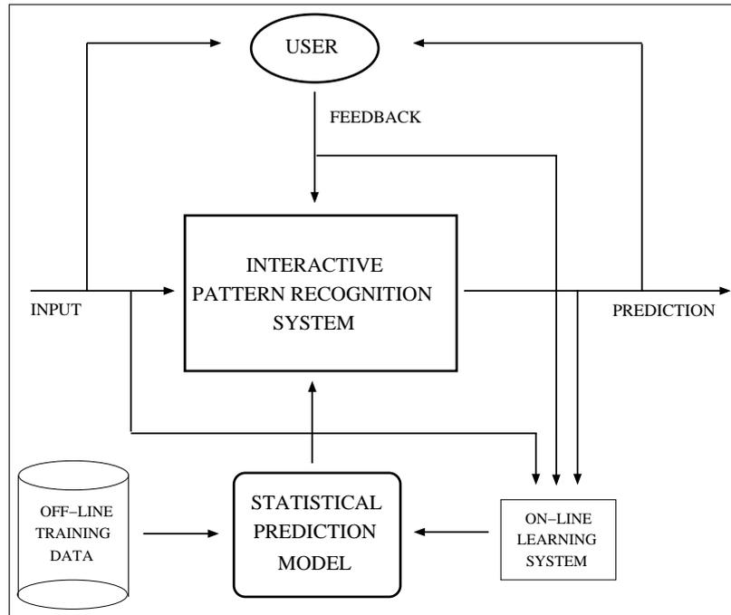
**Figure 2.4:** IPR system incorporating an adaptive learning module.
