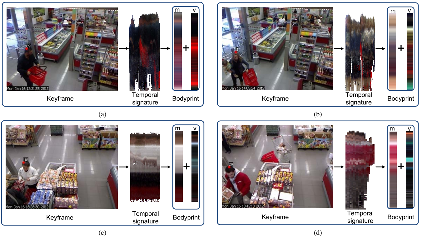
Fig. 2 Some examples of bodyprints. All the examples show different outliers generated by carried objects. Figure c presents missing data in the lower body.
