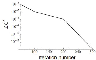
Fig. 10. Cost function associated with the extended coupling matrix from Table VIII, calculated using (15) using the Nelder Mead algorithm. Using (15) we reach a solution while using (13) we fail.
