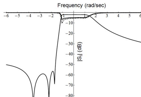
Fig. 2. Target S-parameters for an asymmetrical lossy filter (low-pass prototype with unity source and load resistances) [p. 60 in 20]: solid lines for  $|S_{21}|$  and  $|S_{11}|$ ; dashed line for  $|S_{22}|$ .
