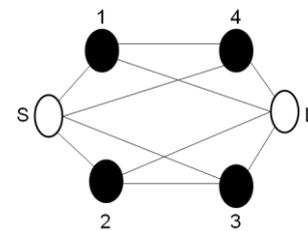
Fig. 9. Parallel coupled filter topology
