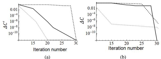
Fig. 7. Cost functions associated with the extended coupling matrix from Table V, calculated using: (a) (15); and (b) (13). (solid line- Nelder Mead, dashed- Simulated Annealing, dots-Differential Evolution)
