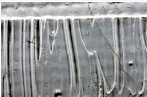
Figura.1 White. Frame no cobalt siccative after ageing for HR and T. A large crack in the paint layer can be observed.
