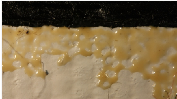
Figura 3. Appearance of oil grooves in the perimeter of the color frames after ageing by HR and T.
