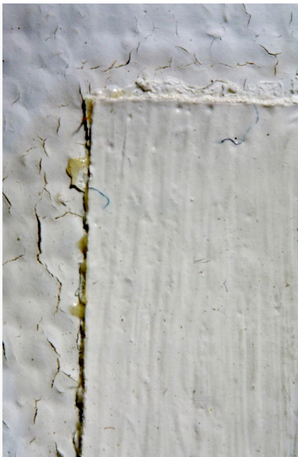
Figura 4. Appearance of oil grooves in the perimeter of the color frames after ageing by HR and T.
