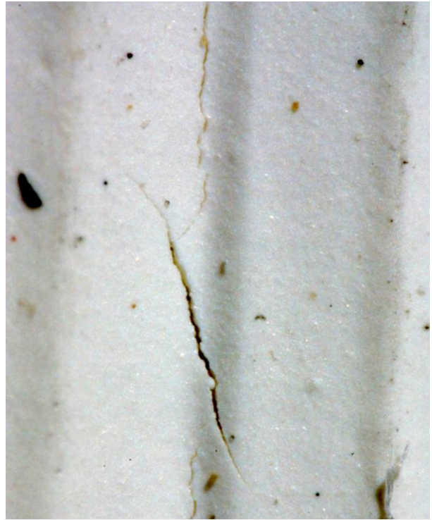
Figura.2 White with 10% siccative. Cracks appear in the paint layer after ageing by HR and T.
