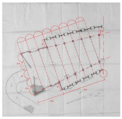
6. Juxtaposition of regulating metric composition on pavilion's floor plan (extract).
