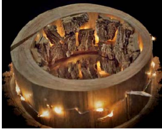
Fig. 2. The inner cavity of Heartwood is lined with micro leds recessed behind bark.
