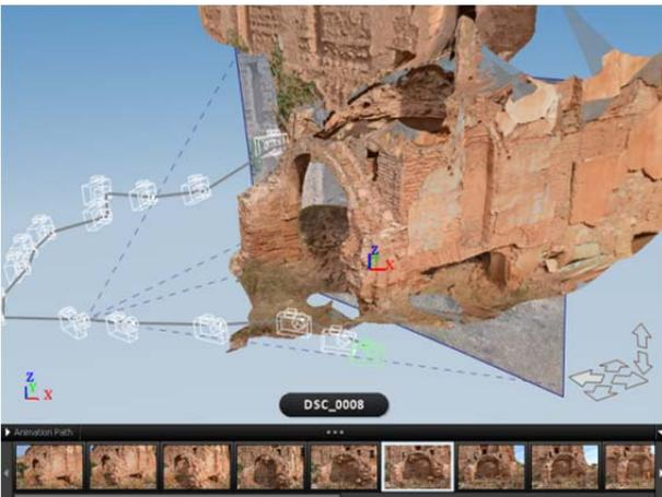
**Figure 12:** Photogrammetric model of the remains of arcs from the cloister made with 15 photographs. In the image it has been marked the different points where pictures have been taken from, which are shown on the bottom sequence.
