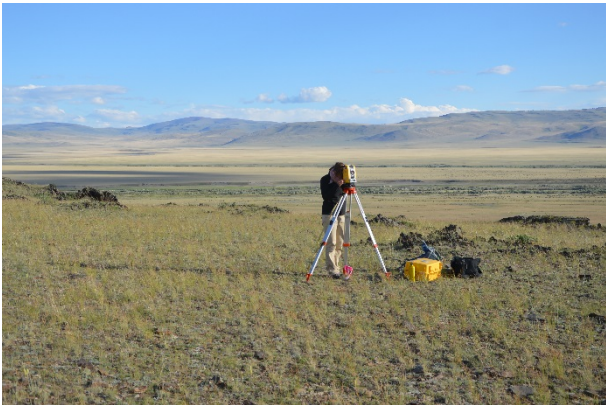
Figure 6: Using a total station to measure the ground control points.
