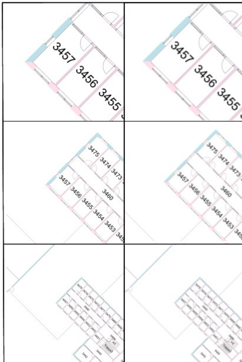
Figure 18. Image quality comparison between SVG rotation and PNG rotation. Sizes of 50, 100 and 200 pixels. Angle of 45°. SVG rotation: left, PNG rotation: right.
