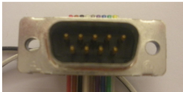
Figure 9. Male RS-232 pinout
