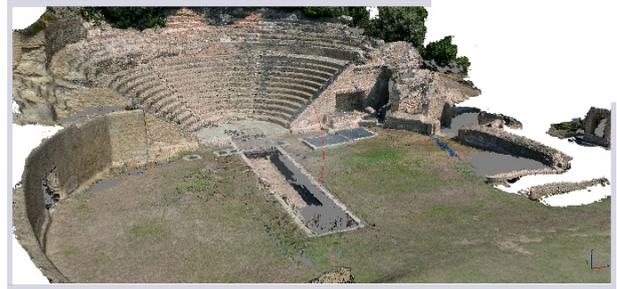
Figure 3: Photogrammetric dense point cloud.
