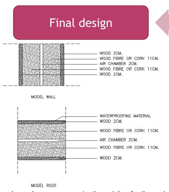
It has been chosen as a constructive solution for the enclosure composite walls of two sheets with a thickness of 28cm. With this enclosure made of wood as outer cladding and cork or wood fibres as thermal insulation is possible to fulfil the requirements demanded by the project. Including theFirestone UltraPly TPO sheet as waterproofing on the roof. This enclosure achieves a transmittance less than 0.15 W / m2K with wood and cork, the most environmentally friendly materials.
