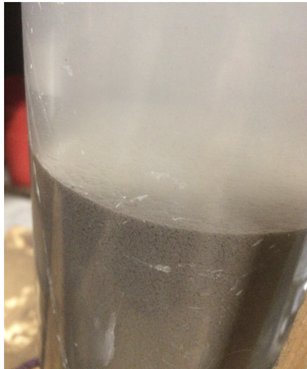
Figure 4.5: Interface in zone settling test
