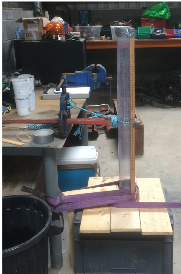
Figure 4.4: Experimental setup for zone settling tests
