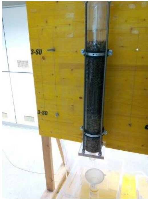
Figure 14. Image of a measurement made during the saturated hydraulic conductivity experiment.
