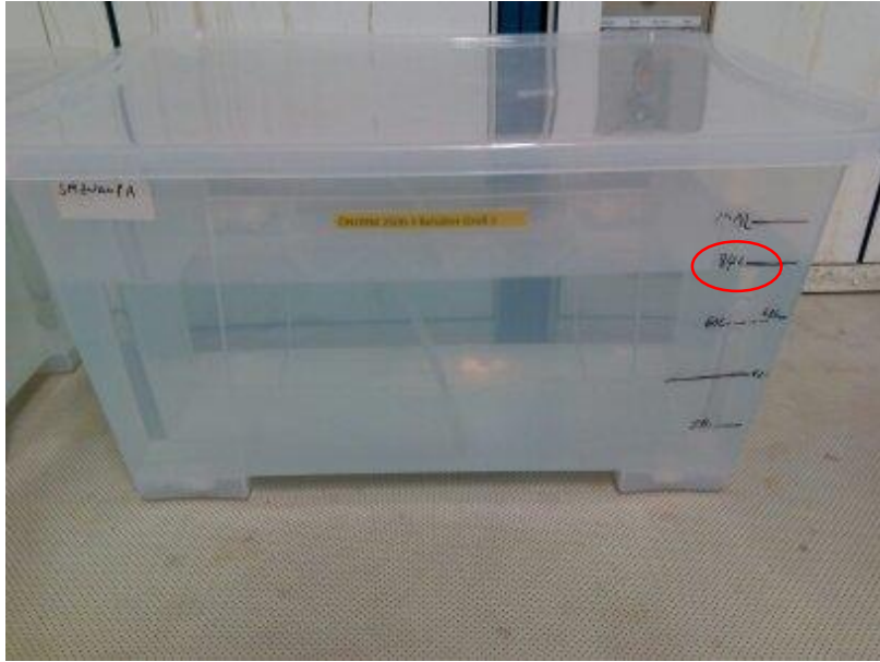
Figure 40. Plastic container used for carrying out the saturated hydraulic conductivity experiment.
