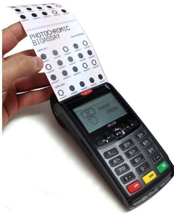
Fig. 5. Exemplary application of a point-of-care bioanalytical system that exploits thermochromic paper and commercial thermal printers.
