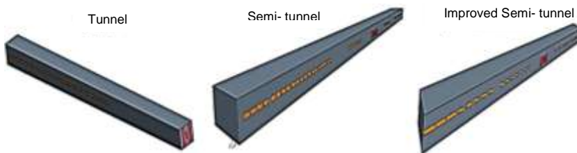
Figure 4.1. Tunnel (T), Semi-tunnel (ST) and Improved Semi-tunnel (IST) configuration. Only half building is presented because symmetry was applied to CFD calculation.
