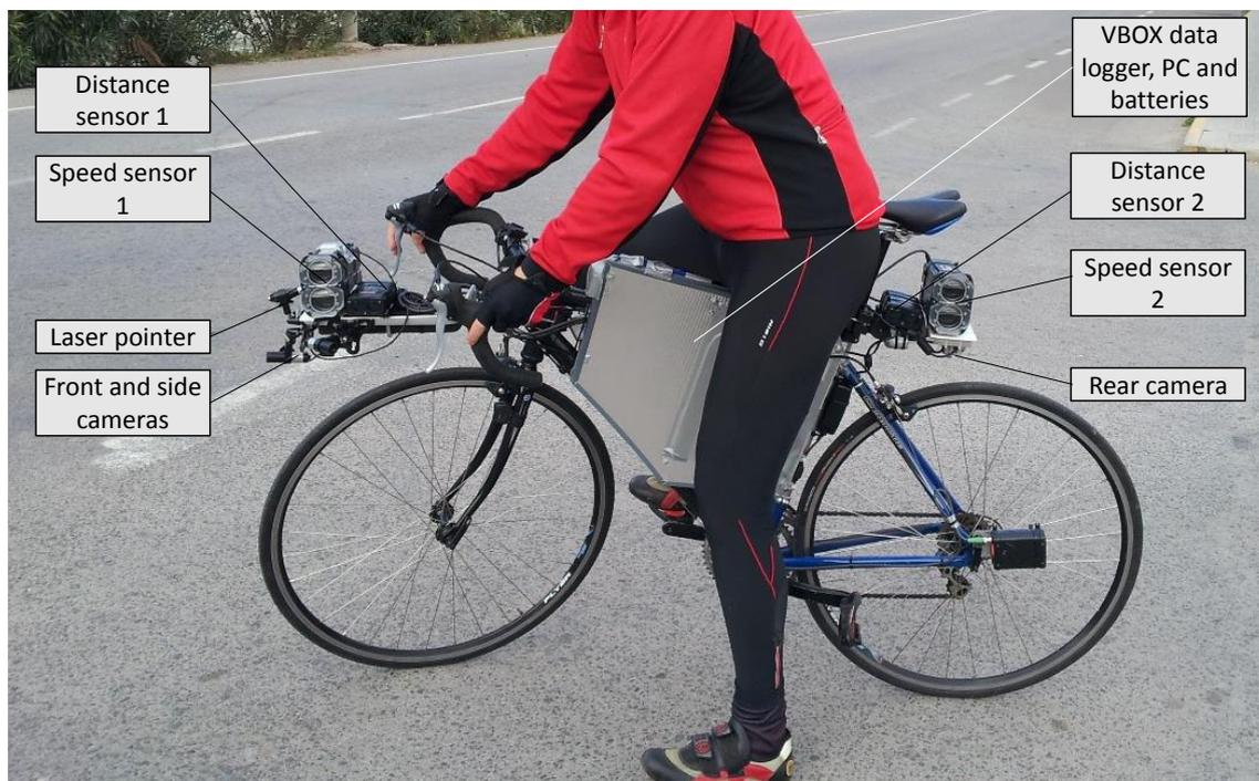
Figure 1. Instrumented bicycle
