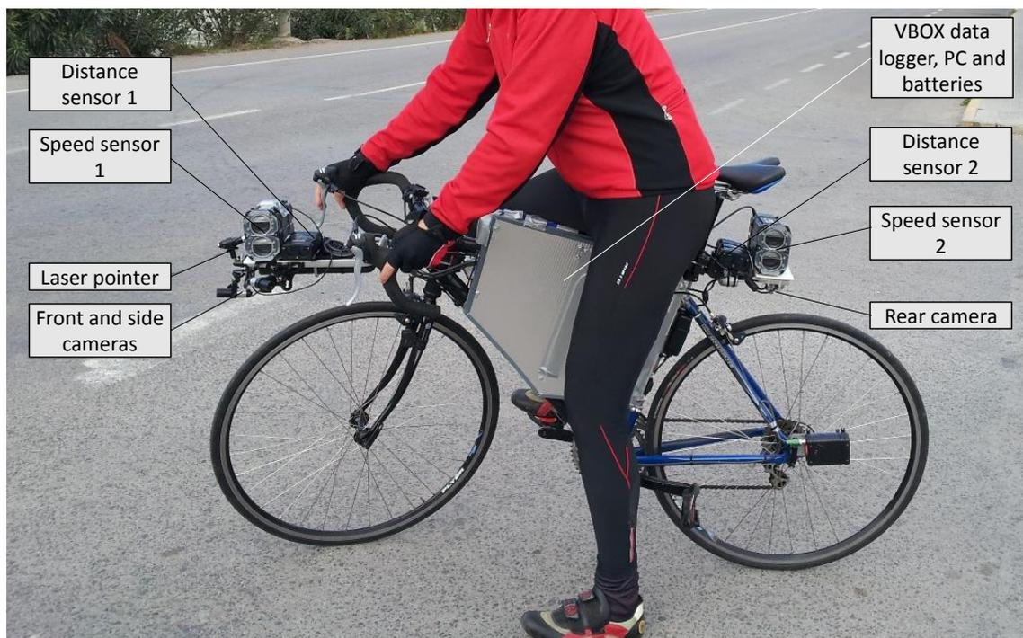
**Figure 1. Instrumented bicycle**
