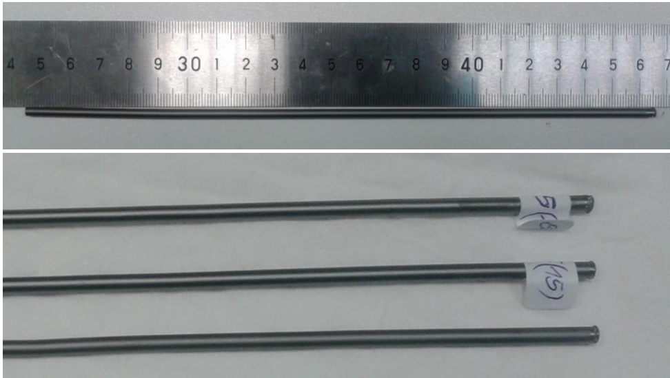
Figure 3.38: BSCF capillaries used during permeation/reaction characterization. Dead end closing detailed in picture below.
