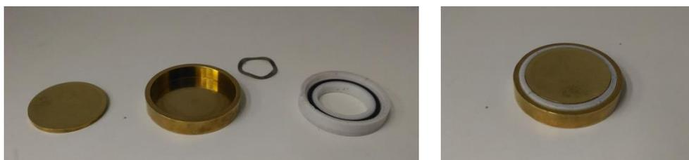
Figure 3.29. *BDS-1308 liquid parallel plate sample cell used for proton conductivity measurements*
