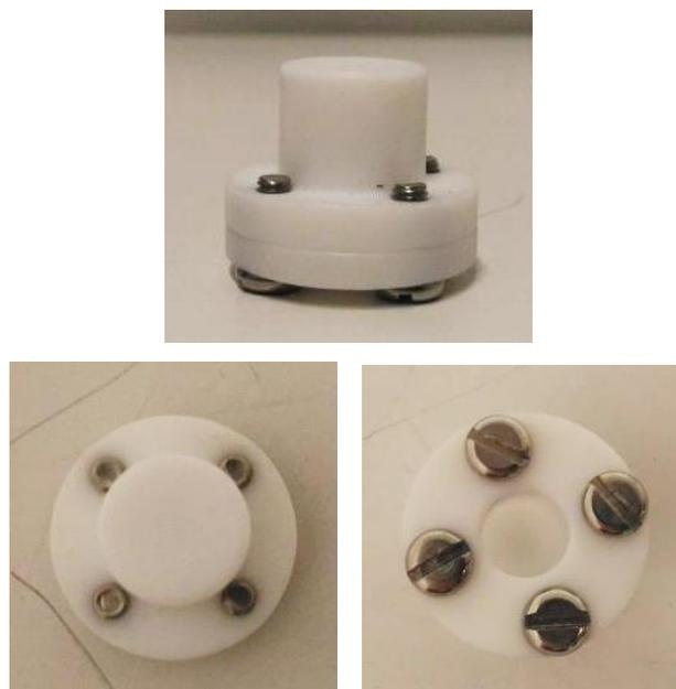
**Figure 3.31. Pictures of the home-made gravimetric cell taken from three different views: front, top and bottom side**
