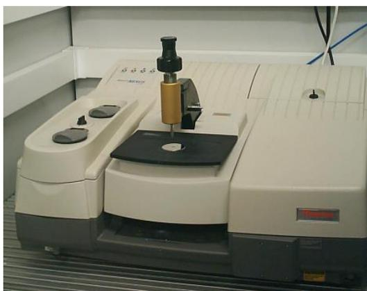
**Figure 3.5. Thermo Nicolet 5700 FT-IR spectrometer**
