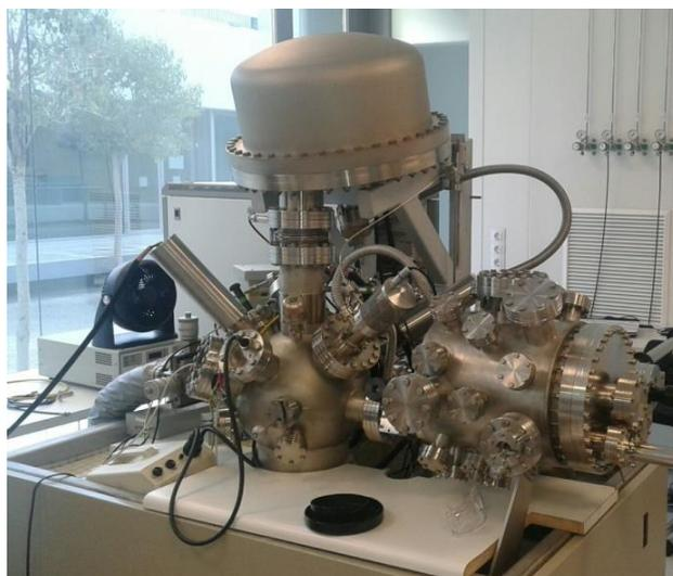
**Figure 3.8. XPS SCALAB 210 multi-analysis system**
