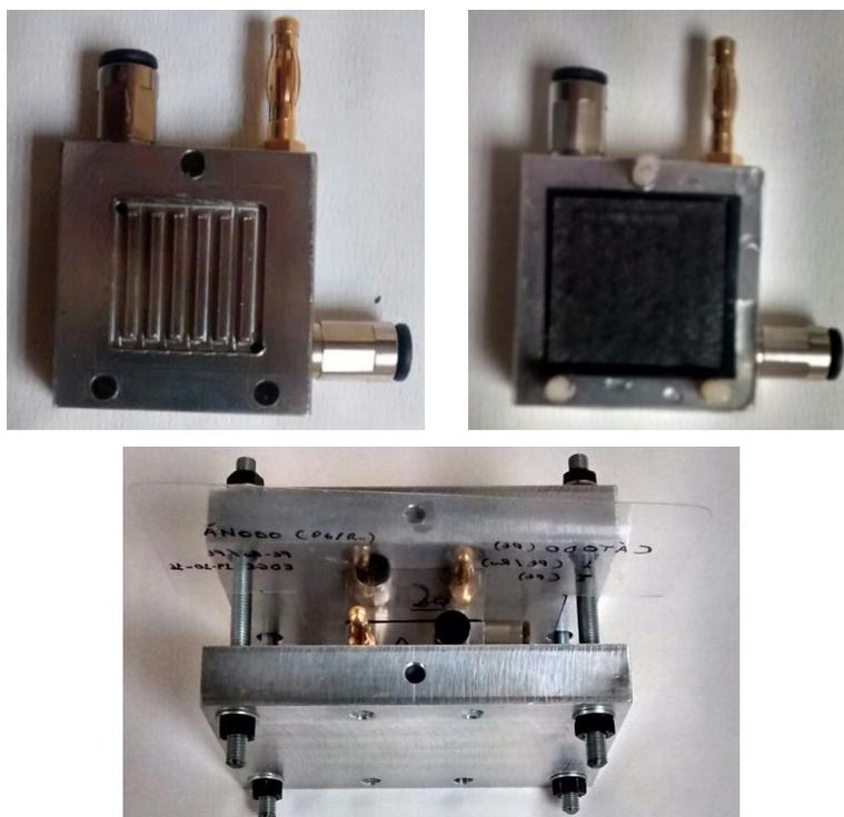
Figure 3.33. Pictures of the single DMFC used to evaluate the performance of the composites
