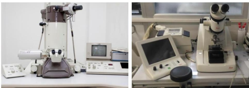
Figure 3.15. *JEOL JEM-1010* transmission electron microscope (left) and ultra-microtome *Leica EM UC6* (right)
