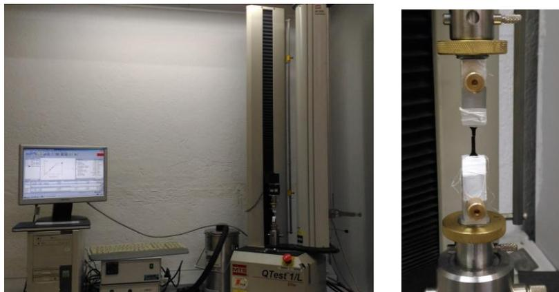
Figure 3.20. *MTS QTest 1/L Elite* Dynamometer (left), and fracture of the specimen after tensile test (right)
