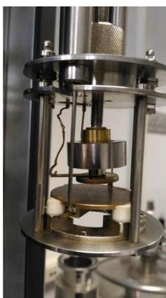
**Figure 3.30.** *BDS-1200 (Novocontrol)*, parallel plate capacitor cell used for the electrical conductivity measurements
