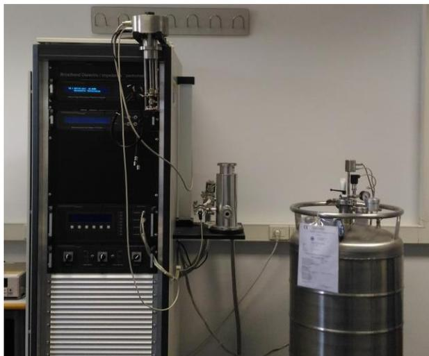
Figure 3.28. *Novocontrol Broadband Dielectric Spectrometer*
