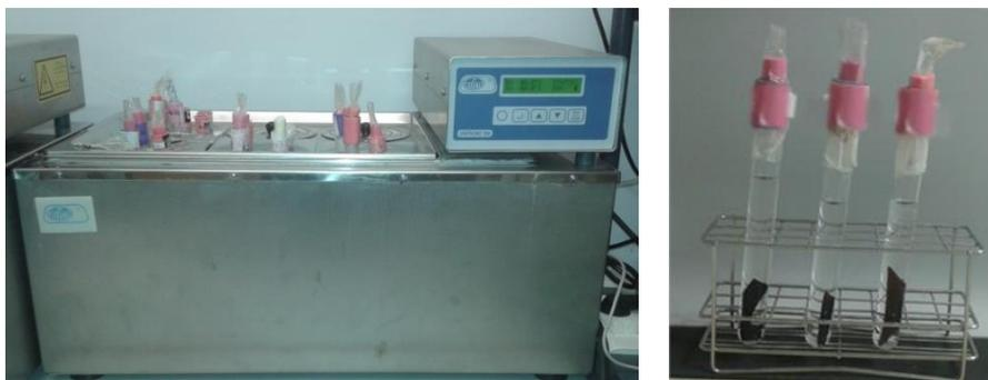
**Figure 3.26.** Isothermal *SELECTA Ultrasonic bath* (left) and a picture of the test tubes with the samples immersed to measure the water uptake (right)
