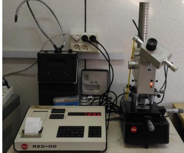
Figure 3.22. Vickers indenter equipped with a *Leitz RZD-DO* microhardness tester
