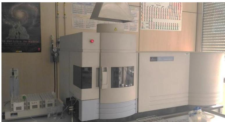
**Figure 3.7. Perkin-Elmer Optima 4300 DV ICP-OES equipped with a spray Scott-type nebulization chamber**
