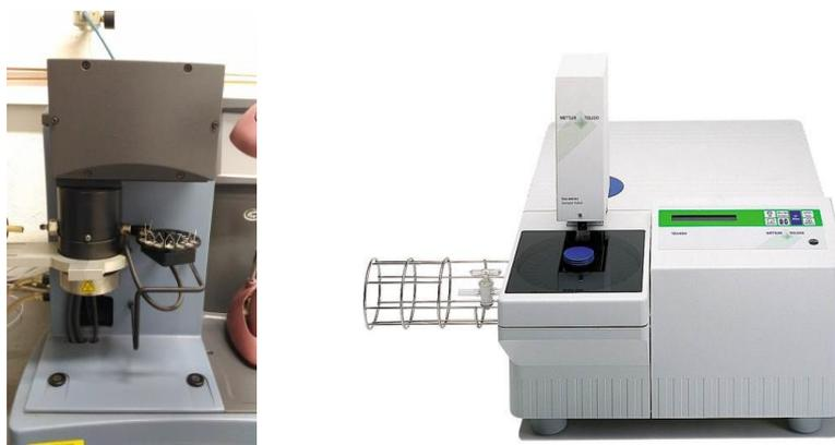
Figure 3.12. *TA Instruments TGA Q-500* analyzer and *Mettler-Toledo TGA/SDTA 851<sup>e</sup> modulus* analyzer
