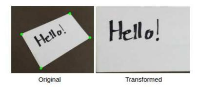
Figure 8.1: Four point perspective transform
