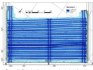
Figure 12: Point density in test area A calculated from the MTLS data (points/m2)
