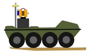
Figure 4: Illustration of the set-up of the survey main components: A) laser scanner, B) GNSS and C) INS
