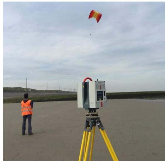
Figure 3: Image based modelling using a kite (KAP)
