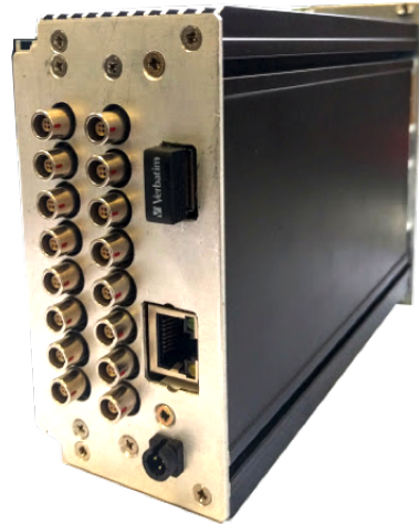
(b) Back side of the device. Output connectors are placed here, together with the USB and ethernet interfaces.
