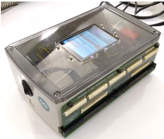
(a) Check system box. All the connectors are placed on the side for easy connection.
