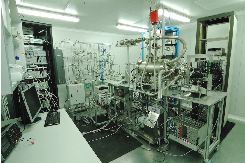
Figure 1.6: The NEXT-DEMO detector and ancillary systems (gas system, front-end electronics and DAQ) in their location at a semi-clean room at IFIC.
