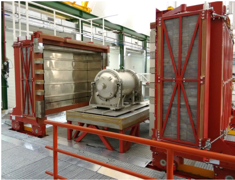
Figure 1.26: The NEXT Experiment lead castle. The NEW detector stands previously to the piping and cabling installation.
