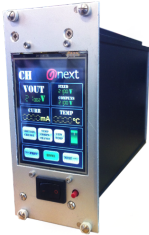
(a) Front view of the bias source, where the touchscreen is placed.
