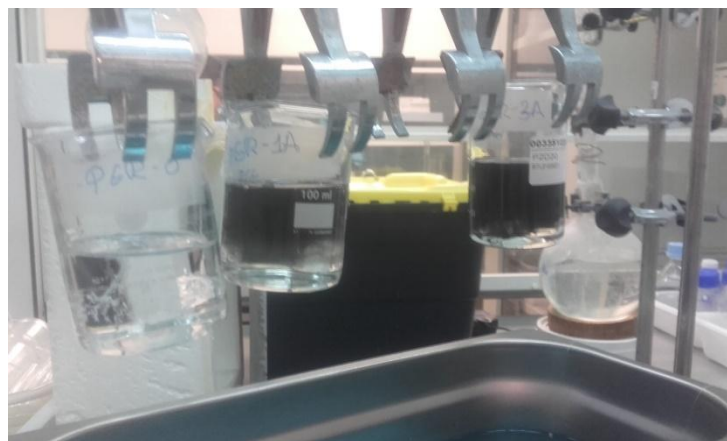
Figure 20. Result of 20 min. of ultrasounding in PCL/GO/Dioxane mixture.
