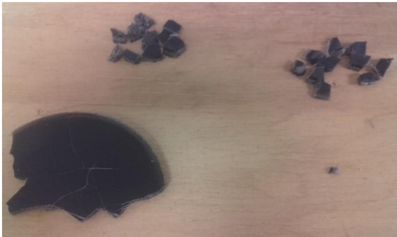
Figure 26. Sample PCL/GO containing 0.5% wt. GO respect to PCL and the smaller samples used for posterior characterization techniques.
