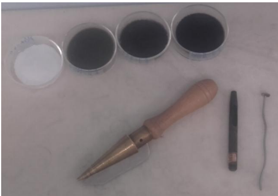
Figure 24. The four samples created (from left to right- 0%, 0.1%, 0.2% and 0.5% wt. GO in proportion to PCL) and the apparatus used to punch the discs from the samples.
