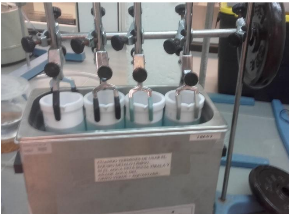
Figure 21. Ultra-sound bath containing four Teflon crystallizers which contained the PCL/GO/dioxane mixture to be sounded.
