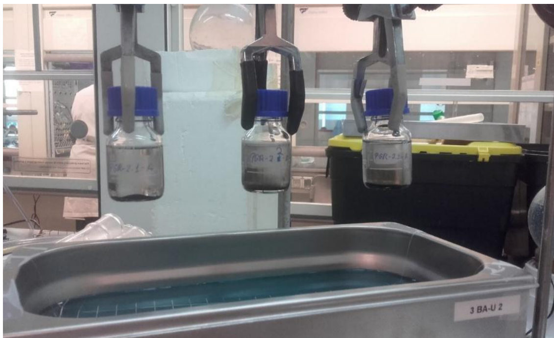
Figure 20. Arrangement of the ultra-sound bath and the containers containing GO and dioxane prior to sounding.
