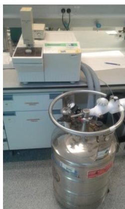
Figure 33. Mettler Toledo 823e differential scanning calorimeter (DSC) equipped with a TSO 801 RO sample robot and cooled with liquid nitrogen.
