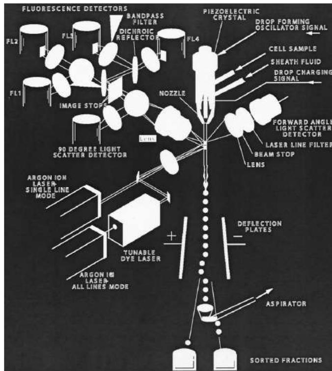
Image 1. Diagram from a Fluorescent Activation Cell Sorting (FACS) machine (Herzenberg, L. A. *et al*)<sup>1</sup>.
